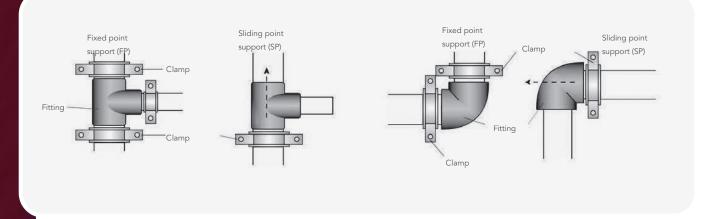
The position of the FP depends on where the pipe expansion absorption devices are located. The distance between the SP depends on the temperature of the fluid. The higher the operating temperature, the greater the expansion. The pipe support clamps are only considered FP's when they are changing direction, opposing the expansion or contraction movement of the pipe. When they do not limit the expansion or contraction of the longitudinal direction, we consider it to be an SP.
